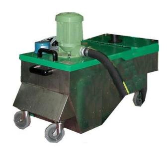
This spray system has an efficient mixing system and its vat is especially conceived to avoid sedimentation. It is essential for magnetic particle inspection equipment.
